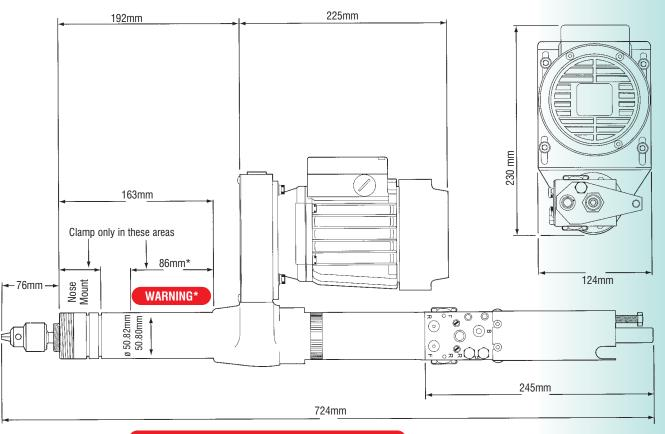
\*Do not exceed 4Nm (3 lbf-ft) clamping torque here.
